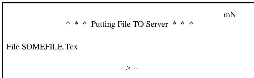
This screen automatically appears in the NFT Session when a PUT operation is in progress. It shows the name of the file being sent to the file server. The activity indicator consists of several dashes with an arrow that slowly moves to the left. When the transfer is completed, this screen disappears.
